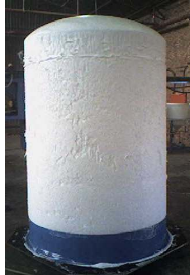
The Cannon Viking Blockmatic is able to produce round blocks for peeling (as above) or standard rectangular blocks for the production of standard, HR and visco foams (as below)
