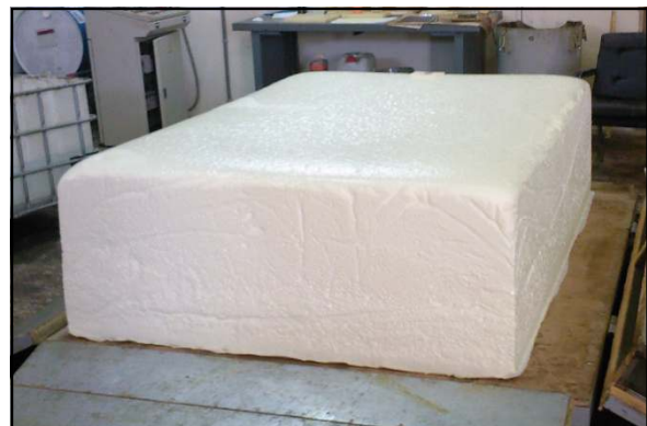
The Cannon Viking Blockmatic is able to produce round blocks for peeling (as above) or standard rectangular blocks for the production of standard, HR and visco foams (as below)
