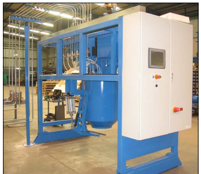
The Cannon Viking Blockmatic complete with HMI PLC Controls undergoing final testing in Manchester before delivery to another customer
